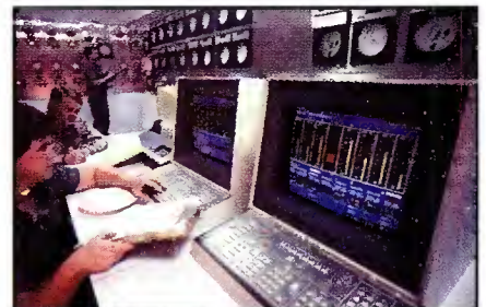
Hundreds of variables in the tape manufacturing process are computer-monitored in this mix prep control room. (Courtesy of Ampex.)
