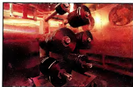
An environmental chamber used for accelerated aging tests of magnetic tape. (Courtesy of Ampex.)
