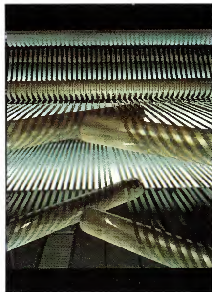
A videotape slitter at work. (Courtesy of Agfa.)
