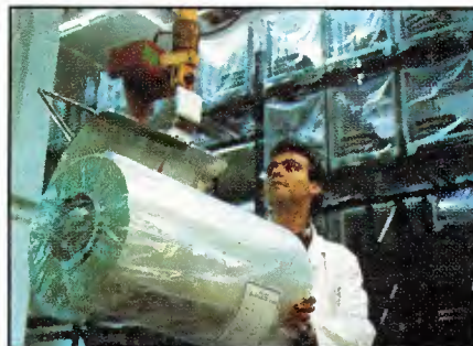
A roll of polyester base film being loaded into machines that will prepare it for coating. (Courtesy of Agfa.)
